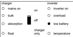
The inverter is switched off due to low battery voltage.
