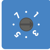
Rotary switch set to position 2
