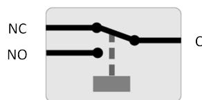
Relay configuration (not energised).
